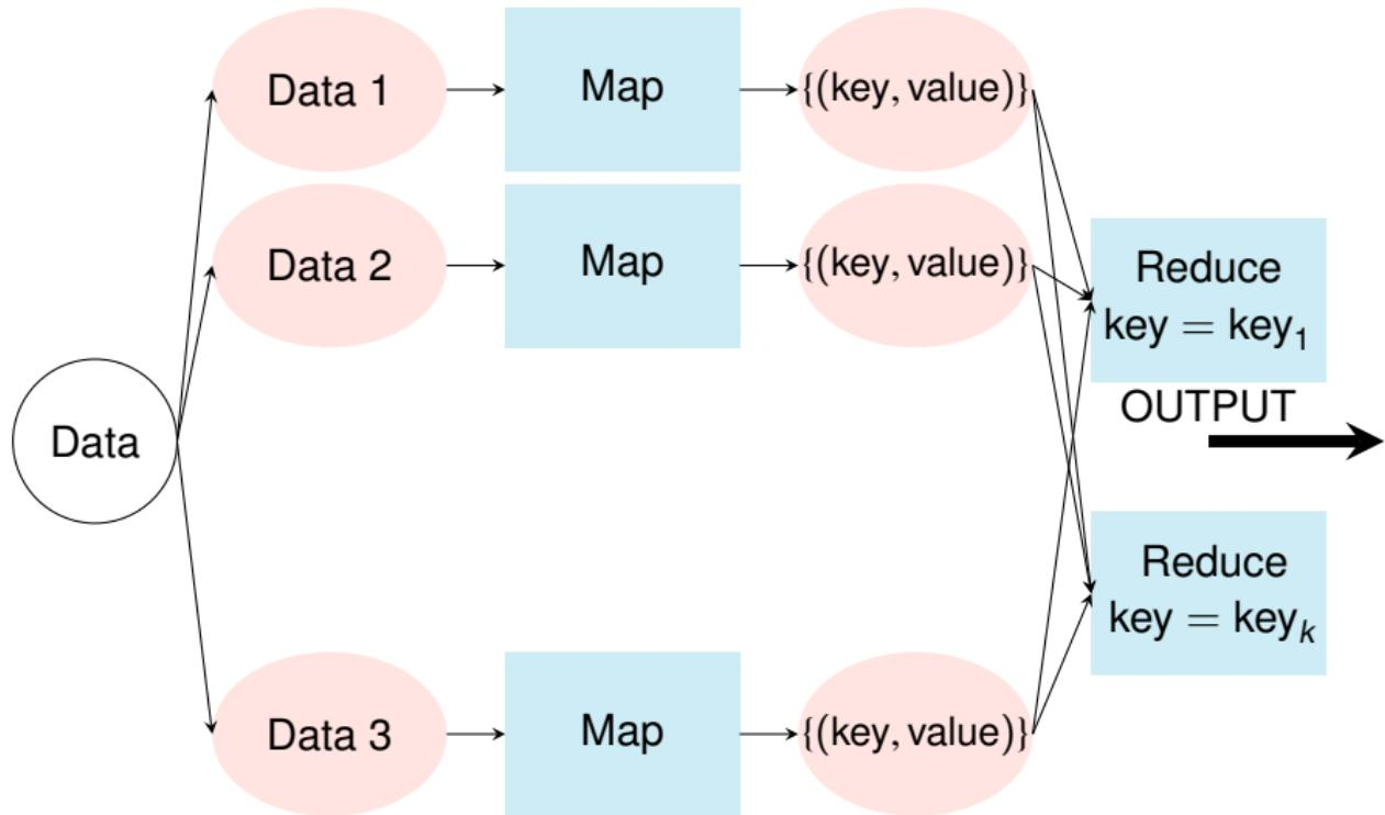
Each key is processed through ONE reduce step to produce the output.
